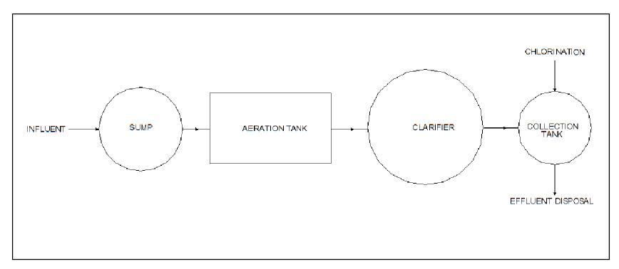
FIGURE 6.4 FLOW CHART FOR EFFLUENT TREATMENT PLANT
