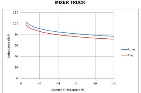
FIGURE 4.1 NOISE LEVELS dB(A) DUE TO CONCRETE BATCH PLANT + CONCRETE MIXER TRUCK
